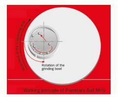
**Figure 1.** Planetary Ball Mill PULVERISETTE 7 *premium line* (*Fritsch GmbH*) and general operating principle of Planetary Ball Mills.
